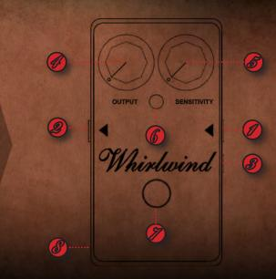
INPUT JACK Connect a cord from your instrument here. Removing the cord from the INPUT jack when not in use disconnects the battery which will prolong battery life.
