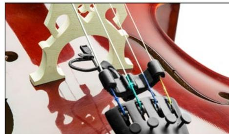
The positioning arm on the I2 Cello Mount allows for a variety of microphone positions, including under the bridge or over the F-hole. Make sure the silver (active) side is pointed toward the body.
