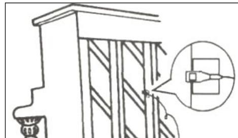
For upright pianos try affixing an I2 Omni to one of the central backposts, as shown. Experiment with placement as not all parts of the soundboard resonate the same. Two mikes in different areas should yield even better results.
