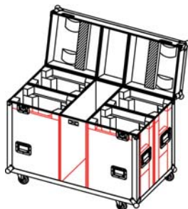
MOVING HEAD CASE 3 Flight case for 4x BTX-SATURN
