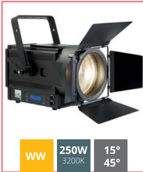
SFX-FR250W Fresnel warm white 250W COB LED projector with motorized zoom
