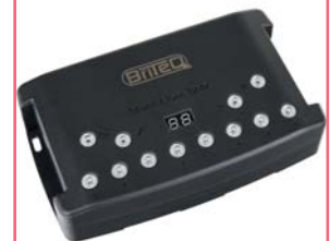
LD-512EASY+ 512-channel DMX interface with 8 buttons. For CHROMATEQ software.
