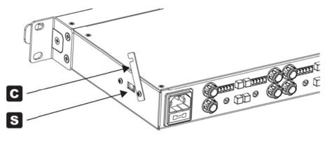
For a qualified technician to change the AC voltage setting, the AC cord shall be detached, the security cover (C) shall be flipped up, and the Voltage selector switch (S) shall be set to the new position. Afterwards, the security cover (C) shall be set back into a protective position to avoid tampering with the switch.
