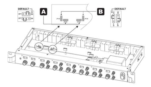
**Emergency Mute.** Jumpers JP102 (for Signal-A output) and JP104 (for Signal-B Output) decide whether the loop-through outputs of the feeding signals A and B carry forward the muting of the signal when a signal become present at emergency input (12). This setting can be useful if the input signal is supposed to be forwarded to a different subsystem, but that subsystem has its own emergency features.
